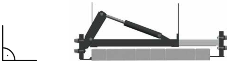
Fig. 16. Adjusting the gripper range: vertical position of the gripper jaw
