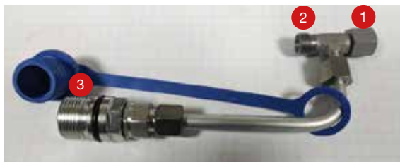
Fig. 62. Blue hydraulic hose connection
