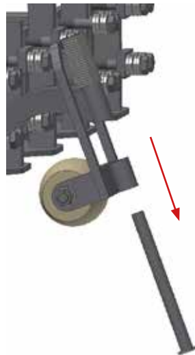
Fig. 27. Pull out the locking pin
