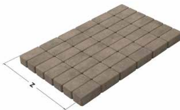
Fig. 13. Adjusting the gripping range: measuring the stone layer
